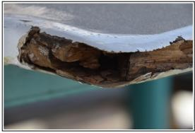
Another job was to repair the hatch of the forward anchor box. Water had found its way inside and the wood was rotten. New wood, micro balloons, glass fibre and epoxi and the hatch was as good as new. It's quite easy to repair a strip plank boat, and not expensive.
