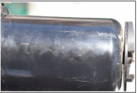
One of our bilge pumps had stopped working so i removed it and took it apart. As you see in the picture the black housing around the electric motor has several cracks. Water has come inside and corrosion has killed the motor. Why the black plastic is cracked I don't know. The pump worked when we left Malaysia a few months ago.
