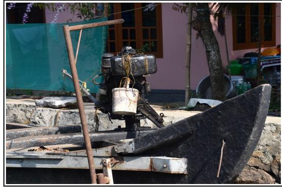
Powering is also very primitive. Longtail drive using engines that seem to be 100 years old.
