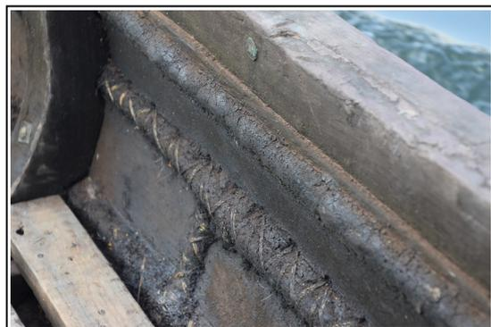
We only saw models of Snake Boats but plenty of other old boat types are still used in the canals. Teak planks are sewn together with coconut fibres to form the hull. Similar technique as used almost 5.000 years ago by the Egyptians.
