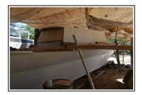
There were many large Bangkas in Port Bonbonon, some were old, even wrecks but there was alo new bangkas being built, in wood, glassfibre and epoxi. The new one on the right picture is about 9 metres long and will do 10 knots with a 45 Hp engine.
