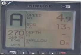
There are many narrow passages between the Philippine islands and the tide can create strong currents. The Hintuan passage is one such place. As you see on the instrumet above, our speed through the water is 4.9 knots while
