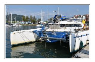
The catamaran on this picture came in the day after us. I talked to the owner and he explained that a fishing boat had crashed right in to the front of him. The beam between the hulls broke and this made the mast fall backwards. So far I understood, but how can a fishing boat crash right into your own boat, front to front? Were both captains sleeping?
