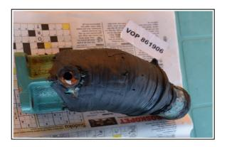
After a few telephone calls I understood that it would take too long time to get a new elbow delivered to Pangkor so I decided to make a temporary reparation and wait until Langkawi where we would have more time. I filled the cracks with epoxi and wrapped the entire elbow up in self vulkanizing butyl tape. Worked fine.
