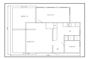
The rebuilding project is planned to span over several years where we use each summer to work with a smaller part. This year we decided to tear down about 1.5 meter of the old house and construct a completely new part two meters longer than the original. This would give us a new sleeping room and a library, totally about 25 square meters of latest energy saving standard.
