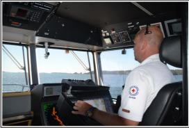
Two big waterjets, controlled by a joystick. Lots and lots of instrumentation on big screens. Captain and mate in comfortable spring mounted chairs.
