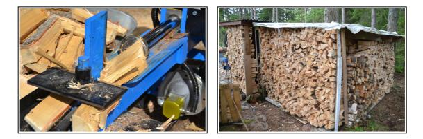
Timber not suited to become planks, I cut to pieces and split into firewood with my new 7 ton Faxe 500 electro hydraulic wood splitter. A little too expensive for my taste but a very nice machine. I'm sure it will last for the rest of my life...
