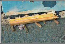
To compensate for this I add 20 cm's to the bottom of the keel. Fixed draft will now be approx. 1.8 meters instead of 1.6. I also move 450 kilos of trim lead that was previously positioned in the aft cabin down to the new keel.
