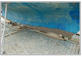
The aft part of the deeper keel in position. The fore part also deepened 20 centimetre.
