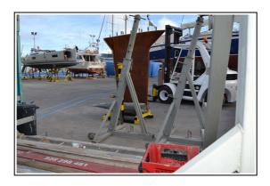
If you look carefully on this picture you see a yacht without keel to the left. The keel rests on the ground behind a grey metal part in the middle of the picture. Check the bulb on the keel. A big part is missing! This French boat was meant to participate in the ARC Race but ran aground close to Las Palmas and was damaged.
