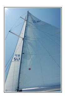
For the first time we could now try our new mainsail. 75 square meters, 5 full battens and MDS-cars all the way up. We also had new propellers. I replaced our fixed propellers during the winter with Volvo Penta Sailprops. I noticed the difference immediately. Much better speed when sailing, specially in light wind.
