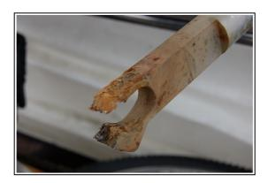
After further investigation we found that the problem was due to corrosion probably caused by the shore power connection. I was well aware of that problem when I built the boat and thought that I had isolated all metal
