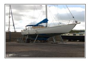
We stayed on land for a couple of weeks, folded the swing keel back into the hull and fixed it in its upper position. To prevent any water leakage we sealed the lower opening of the keel box with plywood and glass fibre with epoxi. We now had a boat with fixed keel and a draft of 1.75 meters. That would have to do for the rest of the season. Finally we also mounted a 2 kW isolation transformer on the shore line input. Better late than never!
