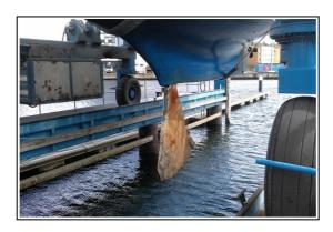
We motored to Ipswich and lifted the boat out of the water. This is what we saw. The hydraulic piston that lifts the swinging keel into the hull had failed and the keel went down with a crash and ended up hanging in the keel bolt/pivot.
