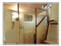
The last ceiling to cover was the ceiling of the deckhouse. Instead of white PVC i decided to use wood for this ceiling. I bought cheap pine boards and coated them with two layers of varnish. In order to make it possible to remove an individual board at a later time i cut away the backside of the groove on each board and then fastened them with a large number of stainless screws.
