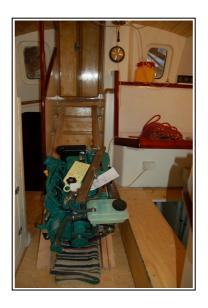
Getting the engines in position was relatively easy. Bertil was first and my old tractor managed to lift him high enough to be able to slide him onto the aft deck. A simple lifting gear, me and 3 strong teenagers and we could move Bertil to the entrance door opening. Down the stairs I let him slide on two wooden planks.
