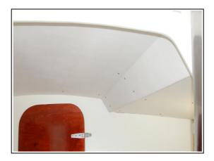
Most of the ceilings are now finished. Covered with PVC film and fastened with stainless screws and washers. This picture shows the ceiling forward of the galley.
