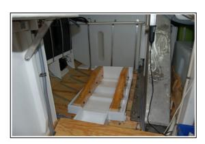
Knowing what motors to fit we could now prepare motor beds in the machine room. A sealed bottom under the motor to keep leaking fluids from spreading into the boat and two well sized wooden beds with 10 degrees of inclination to position the motor in the right angle for the propeller shaft.
