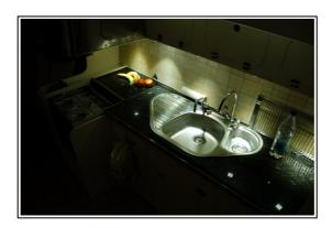
There has also been time to do some job inside. All cabins now have 12 V electric lights. I have spent a lot of time to investigate the possibility of using LED lights but it's still not time to turn to LED 100 % as I see it. Never the less I have installed LED spotlights in the galley. As spot lights, they work well. This picture shows the 5 LED spot lights in the galley. They use only 0.5 Watt each!
