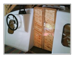
The entrance doors to the deckhouse are finished and mounted. They are made from two pieces of plywood each with 10 mm of heat insulation between and oak frames. The outside is covered with a pattern of wood from juniper.
