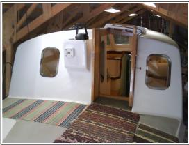
The rudder is now almost finished. Only thing missing is 4 layers of glass fiber and epoxy and that will be done during this winter. Window frames are also finished and mounted.
