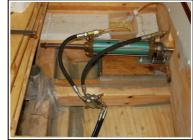
The oil goes from the pump to a bypass and non return valve and further down where it connects with the electric pump for the autopilot system. After that the oil continues aft to the steering cylinder. The thin transparent hoses are temporarily mounted to take care of excess oil during bleeding. Close to the cylinder there is also a cross relief valve set to 78 bar.
