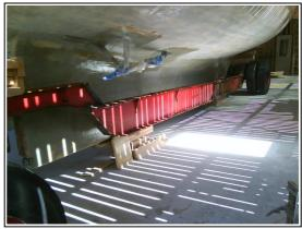
A big job this summer has been the boat wagon. A first test showed that the job I did last summer on the wagon was not enough. Bird of Passage is high, 4.35 meters to be exact and the clearance under bridges is only 4.5. This means that the boat needs to be pretty low on the wagon to pass under. To make that possible I had to lower the frame of the wagon some 25 centimeters.
