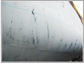
I also have two pictures from a Roberts 53 built in steel not far from here. The owner has used a technique to get a round and nice shape of the hull that I have not seen before. It reminds of the *Radius chine* method but each of the metal sheet parts are twisted and welded in a diagonal pattern along the chine. The left picture shows the boat in full size and the right picture is a
