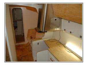
Here is a picture from the galley. The stainless ventilator with it's electric fan over the stove is now mounted.
