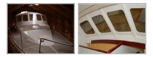
Finally the windows are mounted. Double hardened glass (6+4 mm) for good heat insulation and security. Stainless frames will be added later on the outside.
