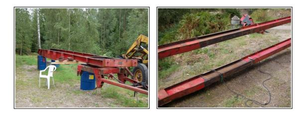
A lot of time this summer has been spent on the old truck wagon. The wheels have been removed to make it possible to remove the suspension and thus lower the wagon about 35 cm. I also need to lengthen the frame 1.5 meters.
