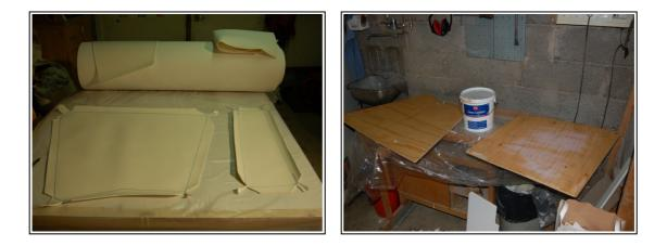
The job now is to cover these plywood sheets with a nice looking PVC film with 3 millimeters of PVC foam on the back side. I use a water based glue from Casco. I have bad experiences from water based glues before so I'm a little bit nervous but I think these glues have become better than they were some years ago. Wish me good luck!
