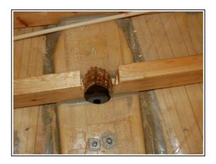
Work with the rudder stock and bearings has begun. Here is the hole in the keelplank for the main bearing.
