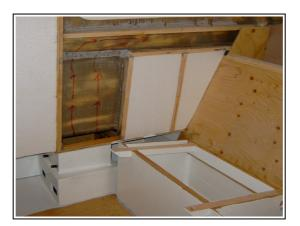
The air passes the heat exchanger and goes vertically up through a channel which continues all the way around 7 of the windows in the deck house. There are 5 windows facing forward and the defroster also takes care of the forward window on each side wall.
