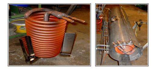
I'm also working with the main heat accumulator tank. It's a complicated construction because I want to be able to heat the water in the tank from electricity as well as the engines and a separate diesel heater. The water in the accumulator tank will heat the convectors in the boat but also produce
