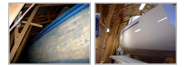
Final painting started in August and continued until the second week in September ! First one side of the hull, white with blue lines, then the next, then the stern, then
