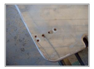
There will be many holes through the deck for fastenings of different kinds. Hinges for hatches is one example. To protect the wood from water coming in through these holes I first drilled larger holes, then filled them with epoxy then drilled the 4 millimeter hole for the screw through the epoxy.
