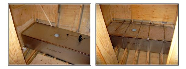
I have been working with fastenings for the water tank in Gustav's cabin. 400 liters of water is 400 kg's of weight. In bad sea the dynamic forces can be considerable, and with time things might start moving. So, I spent a lot of time, maybe too much, to construct strong fastenings.
