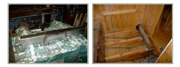
Another job in Gustav's cabin is the mast support. To spread the load I made this beam from stainless steel that rests on 4 floors and takes the load from the mast down into the keel plank and the hull.
