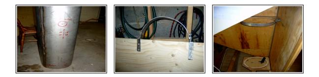
After welding the edges together using his TIG-equipment I marked the positions of all connections with a red pencil. A tank of 120 liters, 1.5 meters high needs good fastenings. I made the metal clamp above to secure the tank properly. The picture to the right shows the clamp in position together with the lower fastening in the machineroom.
