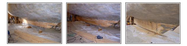
I glued and glued. One layer takes one full day to complete and there are 16 layers to be glued. First picture is 9 layers, second is with 12 layers finished and last picture shows all layers in place. Note the hole for the keel pivot. With the deadwood in place it's time to insert the deadwood bolts. These are made from 12 millimeter diameter stainless steel and positioned in pairs with a distance of 30 cm's. 40 bolts in total, the longest 1.5 meter and most of them around 1 meter long.
