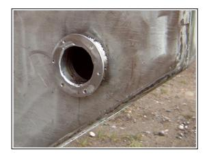
After joining the large pieces I added some small details. In order to make it possible to lift the keel, and then lock it in its upper position and remove the hydraulic cylinder (for service or other purposes) I made a hole in the upper part of the keelbox where i could insert a 75 mm diameter "pin" for the keel to rest on. In order to make this watertight when not used I made a flange with holes for a cover to be screwed on to the flange later.
