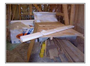
So, with all outdoor jobs finished for this year I started working inside. I now started in the forward cabin, removed all plywood parts, painted them with one layer of epoxi and glued 50 millimeter of expanded polystyrene on the back side of those pieces facing the hull. The reason is heat insulation and floatation.
