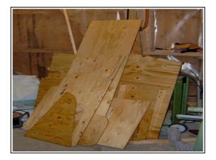
During the winter I will work with the interior. First step is to put one layer of epoxy on all pieces of plywood. There are hundreds of pieces so this will take some time. Each piece is then sanded lightly. Pieces facing towards the hull side are insulated with 50mm polystyrene foam. The roof gets 20mm of insulation. Final surface treatment will vary between different places in the boat.
