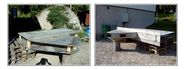
I then placed the two sides on top of each other with wooden blocks between to get the right distance and started adding the remaining side parts. The previous picture shows two of the remaing sides in place, one with a hole for the future hydrualic cylinder responsible for lifting and lowering the ballast keel. By the end of may there is only a few days of welding left, then the entire structure will be cleaned and painted. In june I plan to mount the keelbox in the boat. See you then !
