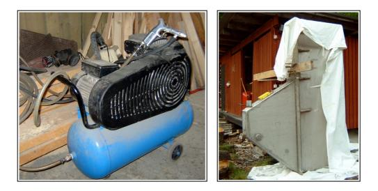
Cleaning the surface of the weldingjoints is important to ensure resistance to corrosion. You can use acid or machine brushing but I chose to try blasting wich worked out well. I used my rather small aircompressor together with a cheap blasting gun from Biltema. By carefully collecting the blastsand and cleaning it I could reuse it several times. The white plastic on the picture was used to keep the sand in the box while blasting the inside.
