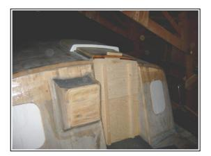
The cold season is here. I have closed the boat, polystyrene foam heat insulation boards in all openings and a temporary door too keep the heat inside. I use a 2.5 kW electrical fan/heater with thermostat. So far it has kept the boat warm and nice without problem.
