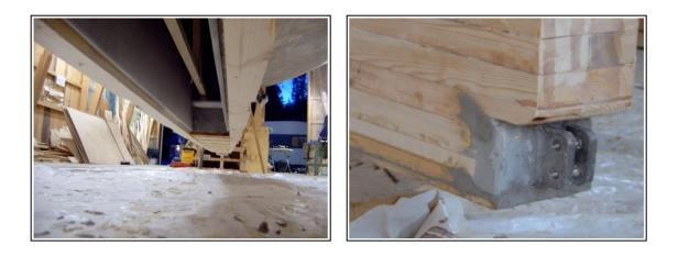
The keelbox is now completely surrounded by deadwood. Above is a picture of the keelbox from inunder looking aft. I aslo added a metal fastener for the lower rudder bearing at the lower end of the aft part of the deadwood. This metal part reaches some 500 millimeters into the deadwood with holes so that 4 bolts pass through it.
