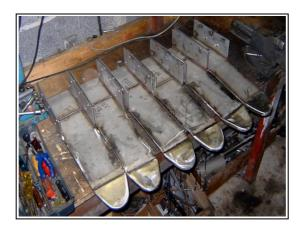
Six chainplates are now almost finished. Missing are only the holes for the turnbuckles.
