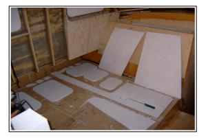
Simple surfaces like the inside of lockers and stowages will be painted with a white acrylat water based paint. White is practical because it makes it easier to see what is inside the locker. The forward cabin will also be painted in some light color, maybe a blue tone with dark blue on the hatches. This picture shows some of the parts being painted and next picture shows one of the junior workers with newly painted lockers in the forward cabin.
