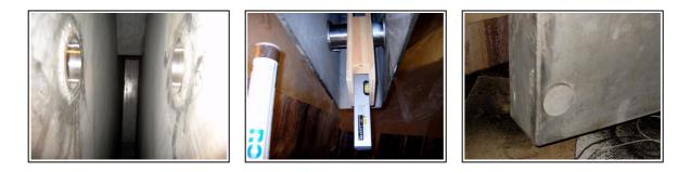
To the left is a view from the inside of the keelbox. To check that the pivot was aligned correctly I fitted my laser level with two pieces of plywood onto the pivot and turned it up and down to simulate the movement of the future ballast keel up and down. The red laser spot moved perfectly in the middle of the keelbox, just as it should. Finally I added the rear support for the ballast keel, a 70 mm solid shaft, also from stainless steel of course.
