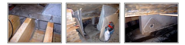
To make the joint between the keelwood and the keelbox waterproof I poured epoxi in between and then added a fillet Once in place there was still some welding to be done on the lower part of the keelbox. To avoid the risc of fire I enclosed the keelbox with plywood, plastic film and old rugs sprayed with water. I then welded on a triangular pivot reinforcement on each side of the keelbox.
