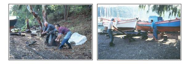
Two guys on the winch pulling up the boat from the water. Then it is moved in to the right position and supported with props.
