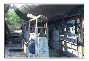
The sleigh is a simple wooden construction with two long boards at the top on which the boat rests. The boards are pressed against the hull by a number of small manual jacks, which are pumped up until the boards follows the shape of the hull. There are more modern shipyards at Preveza but hardly nicer or cheaper.
