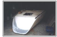
It was now time to continue the work in my workshop. The thin glass fibre shell was removed from the boat and taken inside. See left picture above. I now added a deck (mid picture) and a stern (right picture above). The square opening in the deck was covered by a skylight. I worked most of the winter to complete the extension. To make it stronger I added balsa core inside and a few more layers of glass fibre.
