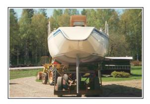
When the weather got warm enough I took the extension outside again and bolted it in position with 20 M8 screws through the old stern. Then some fairing with filler and finally painting with a colour that was as close to the old hull as possible.
