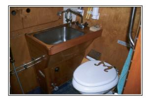
The bathroom includes a large sink for washing, hot and cold fresh water as well as sea water from taps fed by electric pumps. The toilet is a Baby Blake. There was no holding tank installed.
