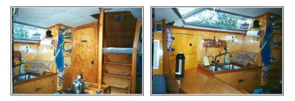
The U-saped galley includes 2 sinks, hot and cold fresh water and an extra tap with seawater. An Origo alcohol cooker with 2 burners on top and one burner in the owen. The entire cooker with owen is mounted on swinging taps and can be used while sailing.
